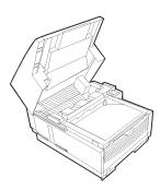
3 Press on the latches on both sides of the copier stacker until the cover of the image drum compartment is released and pops up. Lift up and back, revealing the image drum.
